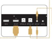
STEP1: Connect one end of a HDMI Cable (not included) to the HDMI ARC port. Cable to the HD OUT/TV port.
