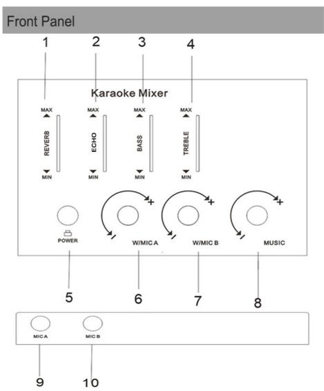
1. POWER / VOCAL CUT (#5): When the receiver is off, short press this button to power on the unit, and the MUSIC knob (#8) will light up blue.
