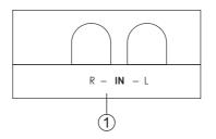
(1) L/R Analog Audio Input Ports: Connect L/R RCA jacks to the audio output ports of audio amplifier, AV receiver, LCD TV, or DVD player.
