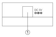
① Power: Plug 5V DC power supply into the unit and connect the adaptor to AC wall outlet.
