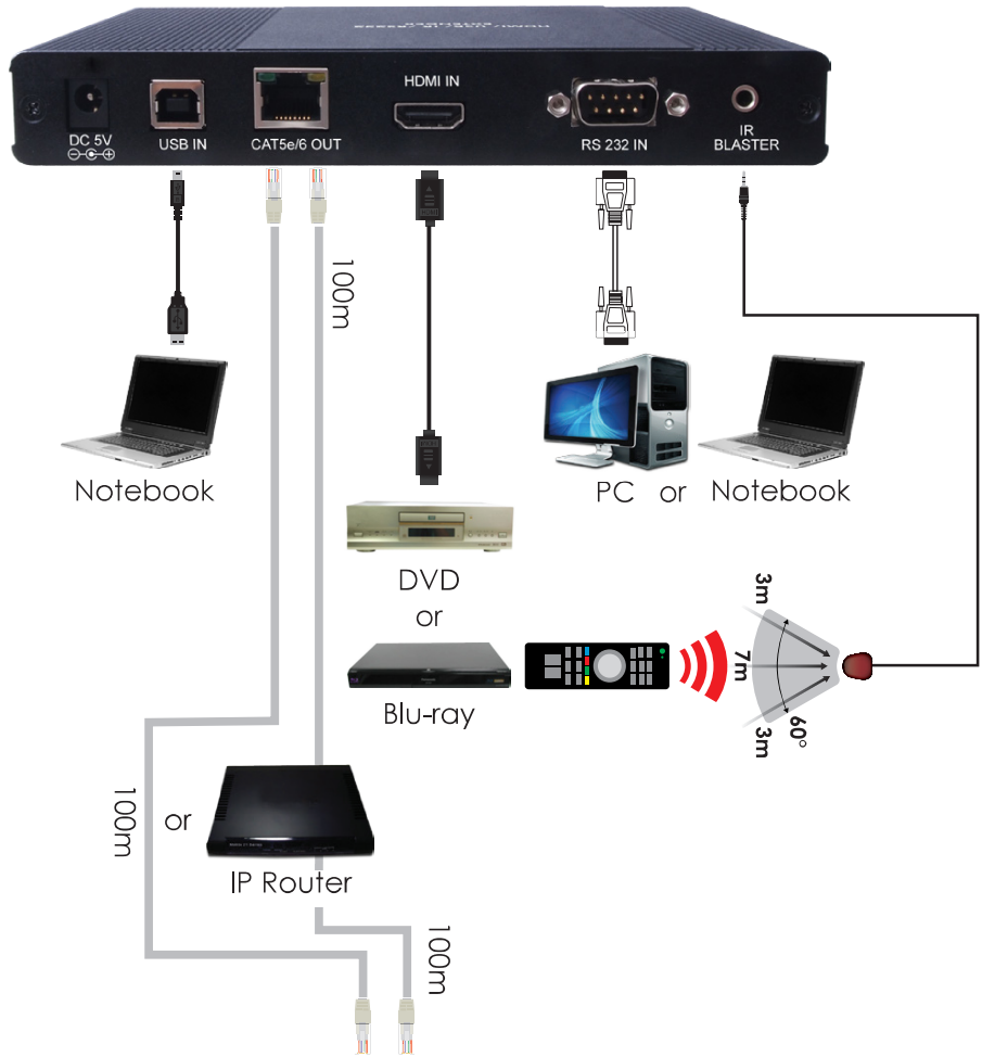
Transmitter's Rear Panel
